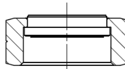
Typ RLF level indicator + Rotalock union nut
